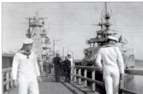
One of the most recognisable features of Admiral Scheer as first constructed was the massive pagoda-style bridge structure. Here, she is tied up in port, moored alongside the old dreadnought Schlesien , her bridge structure instantly recognisable. (Author's collection)
